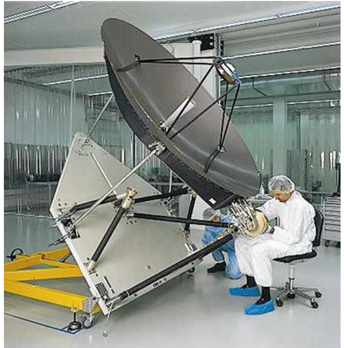
Pyroalliance's equipment on board Rosetta Great Gain Antenna - ESA
